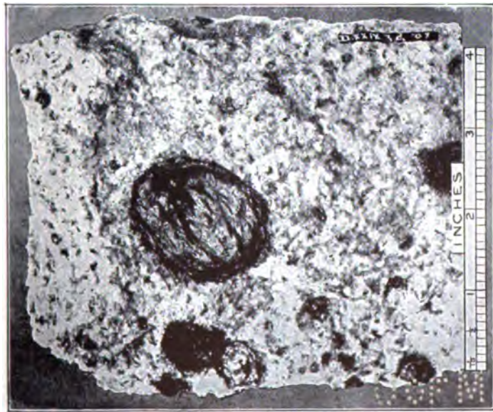
a. Nodular Granite, Ellis Quarry, Bethel. The nodules are mainly muscovite, generally corrugated, and lie with their major axes in the plane of flow structure.
